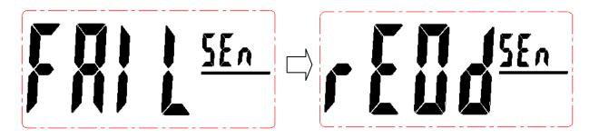
At this time, the SI-100 will redo SPAN Calibration by pressing " $+(\hat{\mathbf{T}})$ " key, will stop the calibration with previous calibration value and go back to measurement mode by pressing " $-(\hat{\mathbf{T}})$ " key.
