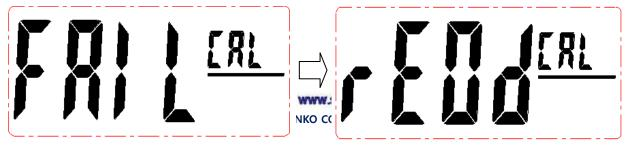
At this time, the SI-100 will redo SPAN Calibration by pressing "+( $\hat{}$ )" key, will stop the calibration with previous calibration value and go back to Measurement Mode by pressing "-( $\hat{}$ )" key.
